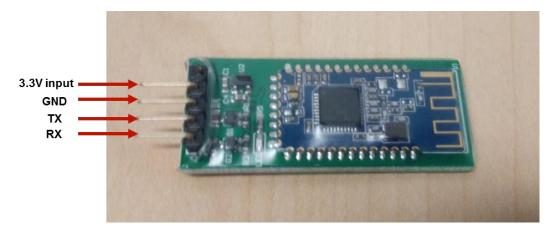
The HM-10 BLE module has two power supply pins, DV33 and DV50. If DV33 is connected to a 3.3V power supply, the TX/RX are 3.3V signals and DV50 should be kept floating. If DV50 is connected to a 5.0V power supply, the TX/RX are 5V signals and DV33 should be kept floating.
