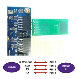
HM-10 BLE modules can be bought from Amazon and Taobo by searching keyword "HM-10 BLE module".
