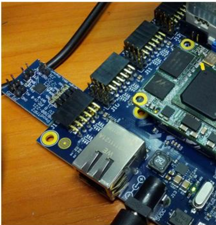
Figure 7 Peripheral Device Connected Using Pmod
