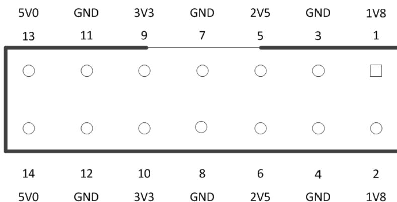
Figure 77 Pinout diagram of the Extension Power Supply connector
