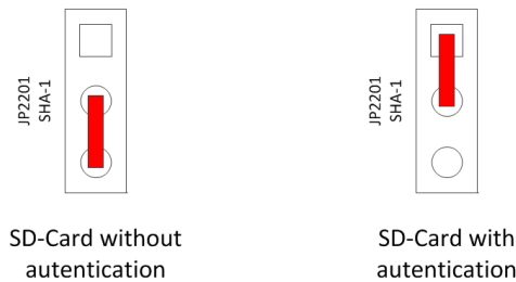
Figure 28 Location of SD-card slot and corresponding jumper
