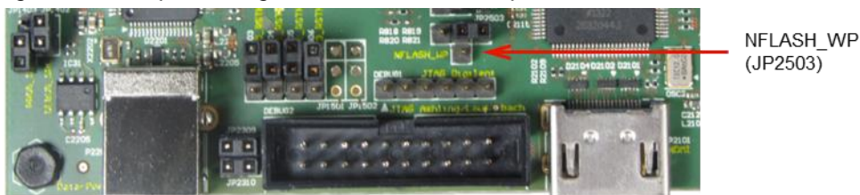
Figure 61 Jumper settings for NAND flash write protection
