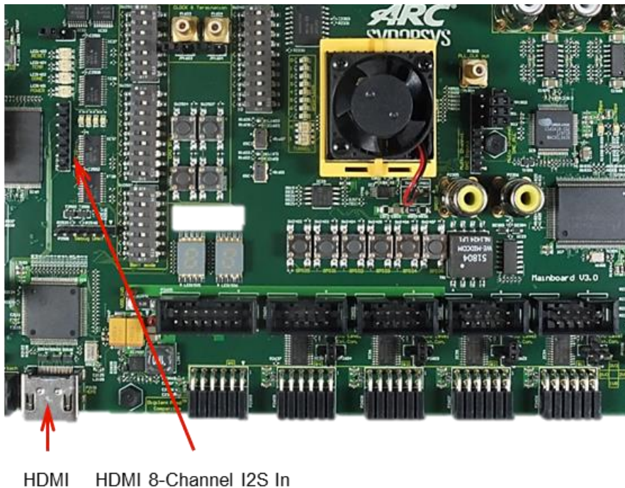
Figure 13 Location of HDMI-related connectors and jumpers on the Mainboard
