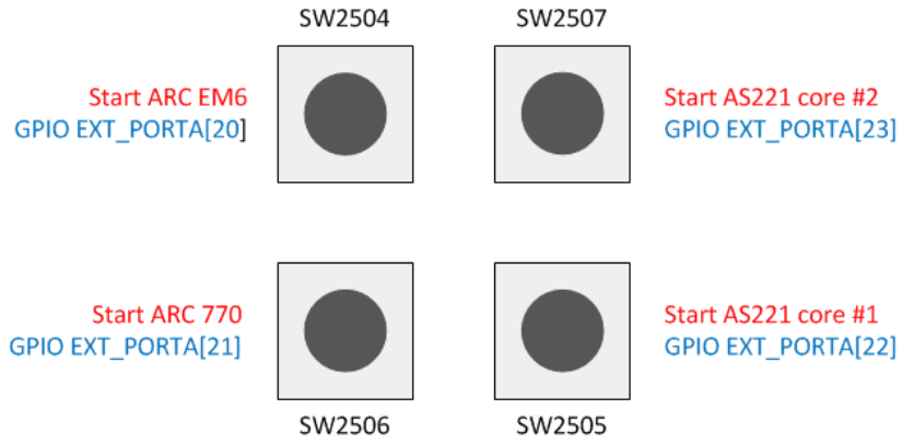
Figure 36 Location of the CPU Start buttons on the ARC SDP Mainboard.
