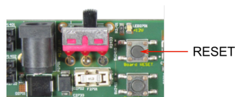
Figure 11 Location of the RESET button on the ARC SDP Mainboard
