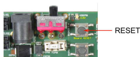
Figure 26 Location of the RESET button on the ARC SDP Mainboard
