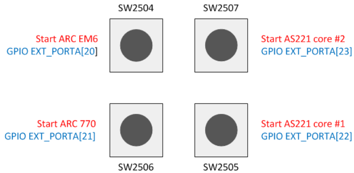
Figure 67 Location of the CPU Start buttons on the ARC SDP Mainboard.
