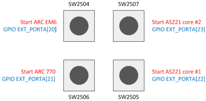
Figure 51 Location of the CPU Start buttons on the ARC SDP Mainboard.
