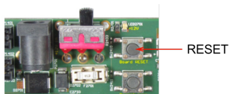
Figure 16 Location of the RESET button on the ARC SDP Mainboard
